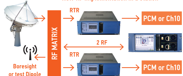
RSR-RF implementation in a station
